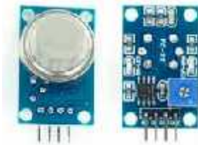
Gambar 3. Modul sensor gas/asap MQ2
